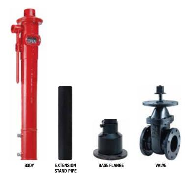
The Indicator Post with gate valve provides a means for operating a buried or otherwise inaccessible gate valve to controlled flow of water in buried pipe. A wrench is provided to fit on top of the unit for turning the gate valve open and shuf
