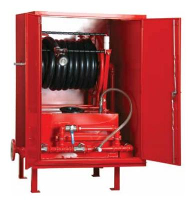
This hose reel station is complete with 1-1/2"  $\times$  30M rigid hose, 225L AFFF foam, stainless steel foam concentrate storage tank, 95GPM foam inductor and nozzle. A bypass loop is provided for water or foam discharge.
