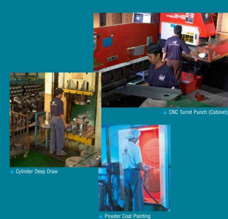
SRI's modern facility allows the company to manufacture high quality hose reels, hoses, fire extinguishers, and cabinets by using advanced computer aided manufacturing methods, a CAD/CAM operated sheet metal machine, automated paintshop for surface pre-treatment and powder coat painting.
