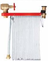
SRI's hose rack assembly is located inside buildings at the wet or dry riser outlet. It features a rack in which hangs the layflat fire hose (30m). An automatic release mechanism allows water to flow through the hose after removal of the hose and nozzle. The rack is available in sizes of 1-1/2" and 2-1/2". There are two methods of mounting the hose rack. One is by using a wall bracket and the other is by fixing on to a right angle valve.
