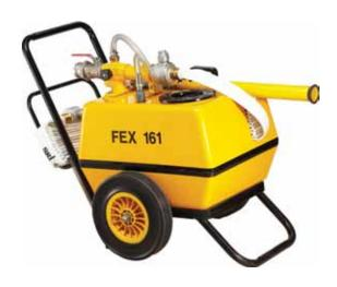
The foam liquid extinguisher on trolley is highly manoeuvrable and it is suitable for outbreaks of fire that cannot be dealt with by using portable extinguishers. It is effective on flammable liquid fire. This is a self-contained foam production unit which only requires connection to suitable water supply (minimum water supply required is 180 LPM at 5 bar).
